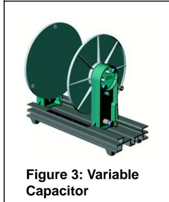
**Figure 3: Variable Capacitor**
