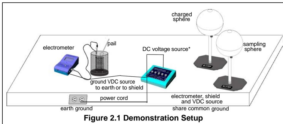
\*An earth ground for the system is obtained through the DC voltage source wall-mount power.
