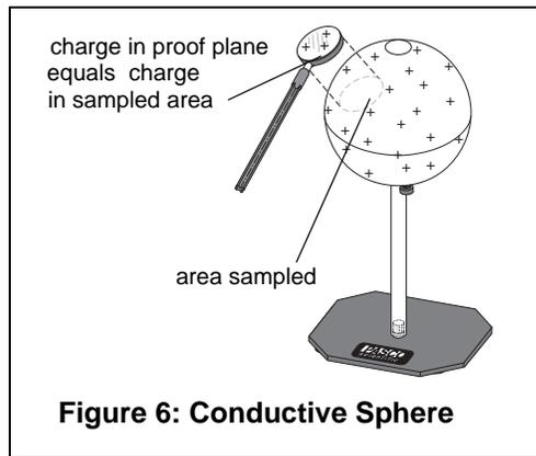
When a proof plane is touched to a conductive surface, the proof plane becomes part of the conductive surface. If the effect on the shape of the surface is significant, the sampling of the charge density will not be accurate. Therefore, always touch the proof plane to the conductor in such a way as to minimize the distortion of the shape of the surface. Figure 7 shows the recommended method for using the proof plane to sample charge on a conductive sphere.
