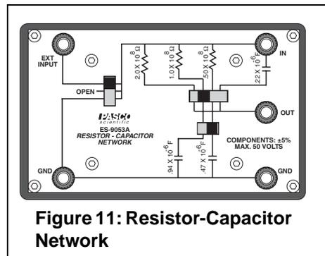
**Figure 11: Resistor-Capacitor Network**
