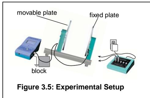
4. Carefully increase the separation of the plates until it is enough to insert the dielectric without forcing it. It should be enough so that you can simply lean the dielectric sheet against the stationary plate. Make sure the dielectric you are using is free of residual charge before inserting it.
