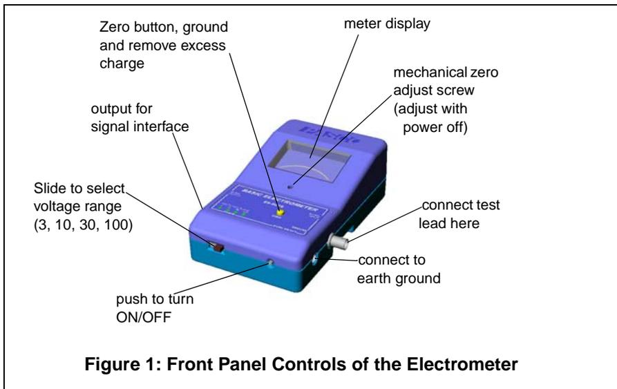
The electrometer is powered by four AA-alkaline batteries, easily replaced by opening the back casing of the electrometer. One of the front panel range-indicator LEDs will blink slowly when the batteries need to be replaced. When replacing batteries, do not touch any of the components or wires in the integrated circuit panel, since they are all static sensitive.
