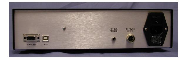
Figure 7. Rear of electronics box. The communications ports are on the left. Use only one.
