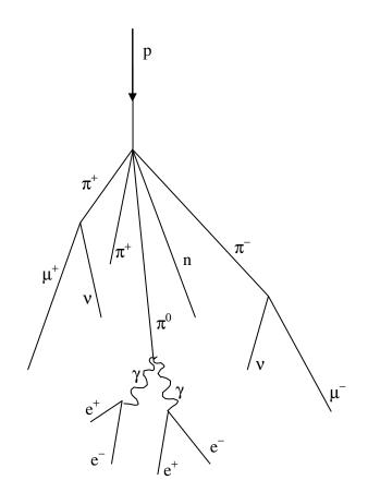
**Figure 1**. Cosmic ray cascade induced by a cosmic ray proton striking an air molecule nucleus.
