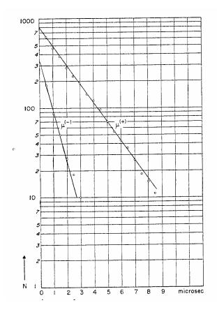
**Figure 3**. Disintegration curves for positive and negative muons in aluminum. The ordinates at t = 0 can be used to determine the relative numbers of negative and positive muons that have undergone spontaneous decay. The slopes can be used to determine the decay time of each charge species. (From Rossi, p168.)
