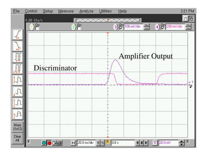
**Figure 10**. Amplifier output pulse from the input signal from figure 9 and the resulting discriminator output pulse. Horizontal scale is 20 ns/div and the vertical scale is 100 mV/div (amplifier output) and 200 mV/div (discriminator output).
