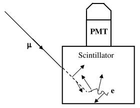
**Figure 2**. Schematic showing the generation of the two light pulses (short arrows) used in determining the muon lifetime. One light pulse is from the slowing muon (dotted line) and the other is from its decay into an electron or positron (wavey line).
