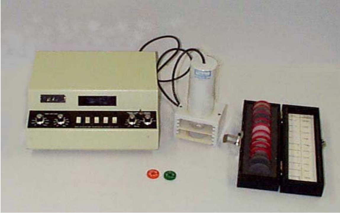
Figure 10. Apparatus and setup for performing the attenuation of radiation experiment.
