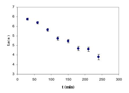
Note that that the error in the large-time (low-count) data is much larger than for the lowtime points. These points will not be weighted as heavily in our least-squares fit: Recall that the  $\chi^2$  which we minimize weights each point by the reciprocal of that point's variance. Points with small error are weighted more heavily than those with large error. The following table gives an idea of the various data point's relative importance to the fit:
