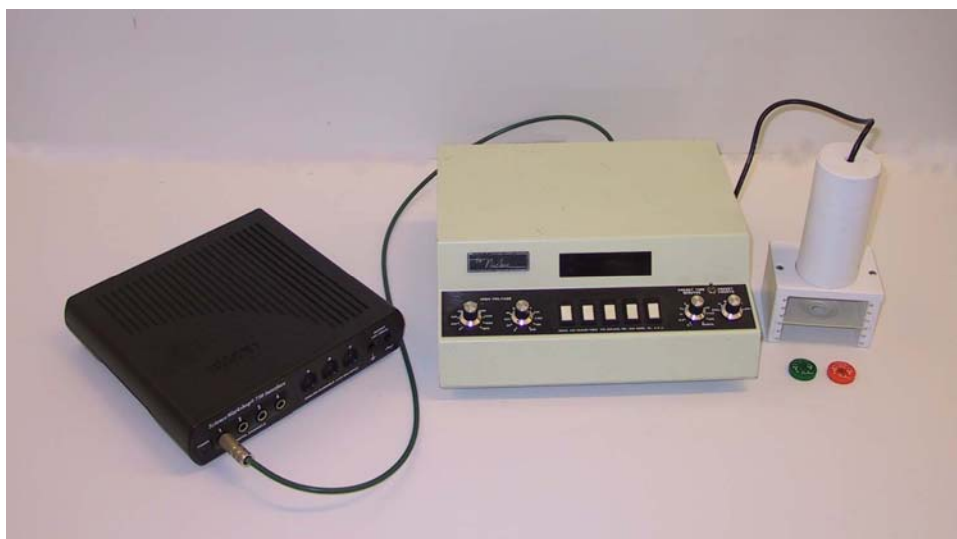
Figure 1. Apparatus and setup for performing the Poisson Statistics experiment.
