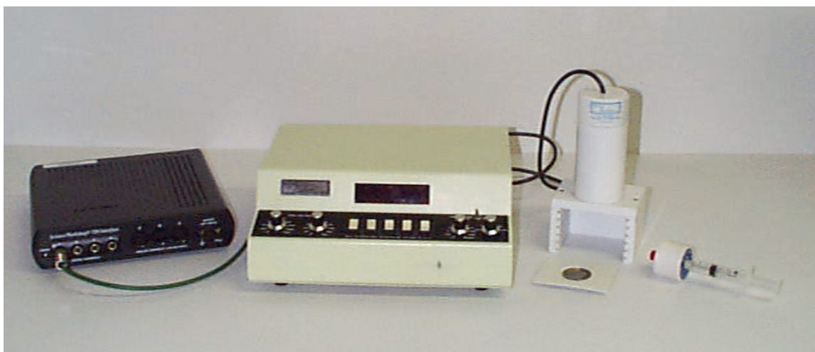
Figure 1. Apparatus for measuring the half-life of Ba-137m.
