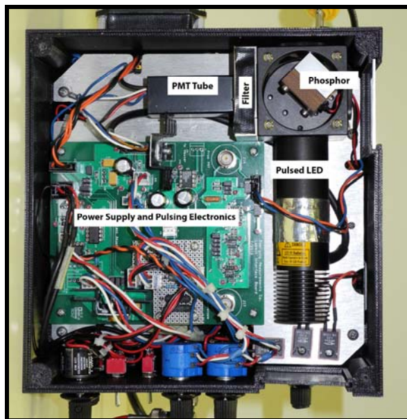
Figure 11. View of layout of components of EMCO LabKit.
