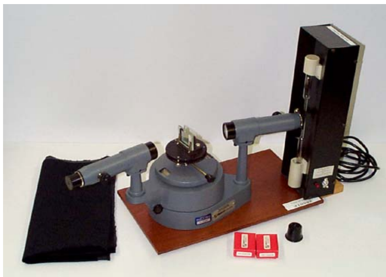
Figure 1. Apparatus and setup for the Balmer series experiment.
