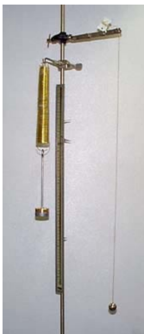
Figure 1. Apparatus for Hooke's Law experiment.
