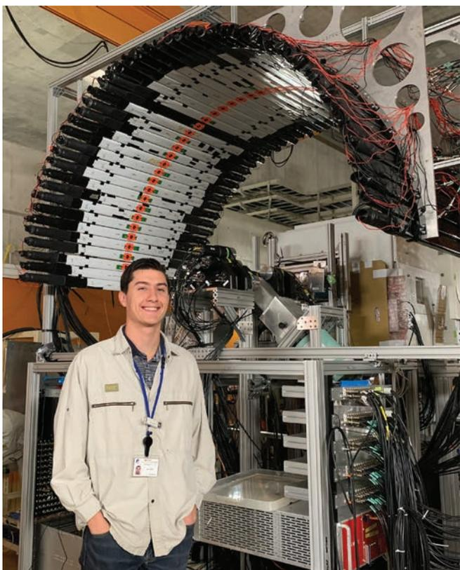
Ian Cox with the VANDLE (Versatile Array of Neutron Detectors at Low Energy) array at the RIKEN Radioactive Isotope Beam Factory in Japan.
