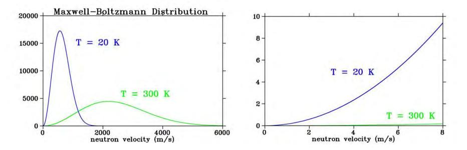
Practical limit for true moderator is about 20k which gives a density increase of ~x20 Practical Thermal Source Limit for UCN production:  $\rho_{UCN} \approx 2 \cdot 10^3 cm^{-3}$
