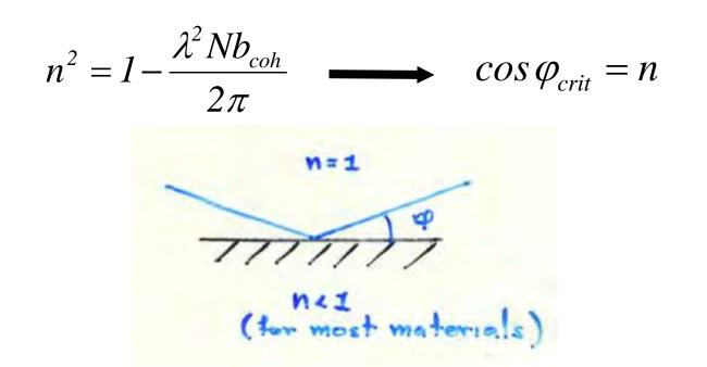
For sufficiently large neutron wavelength,  $\lambda$ , n=0 and  $\cos\varphi_{crit}$  =90°
