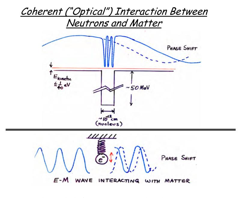
Phase shift leads to Index of Refraction
