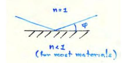
Neutrons will undergo complete "external" reflection from a polished surface for most materials
